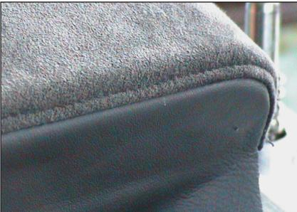
Large Parts, Such As This Leather Instrument Panel, Are Cost Effective To Manufacture With This Process.
